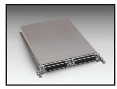
The Model 7703 plug-in module offers 32 channels of 2-pole or 16 channels of 4-pole multiplexer switching that can be configured as two independent banks of multiplexers. The non-latching reed relays provide high speeds and are designed with 300 volt, 500mA; 10VA. The relay closures are stored in onboard memory. The Model 7703 is ideal for RTD and thermistor temperature applications.
